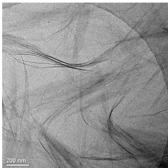
Figure 7. Cryogenic transmission electron microscope (cryo-TEM) images of saturated DSBNI (aq) solution. Wormlike micelles with diameters of \sim 5 nm are observed.
